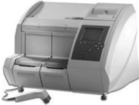
FIGURE 9.13 The Mini VIDAS ® automated system for the screening of pathogens. (Photo courtesy of bioMérieux, Inc., www.biomerieux-usa.com . With permission.)
