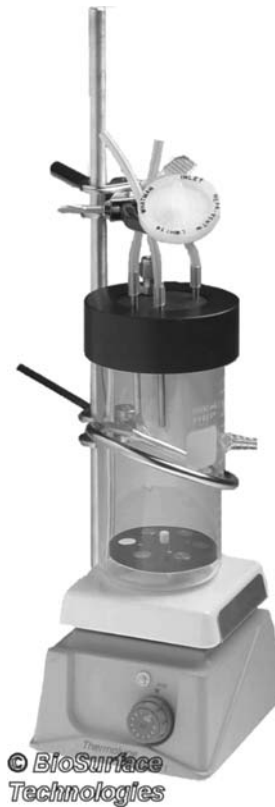
FIGURE 10.7 The rotating disc reactor. (Photo courtesy of BioSurface Technologies Corporation. With permission.)
