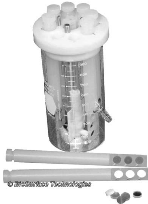
FIGURE 10.9 The CDC biofilm reactor. (Photo courtesy of BioSurface Technologies Corporation. With permission.)
