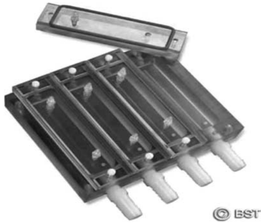
FIGURE 10.6 The drip flow biofilm reactor. (Photo courtesy of BioSurface Technologies Corporation, Bozeman. With permission.)
