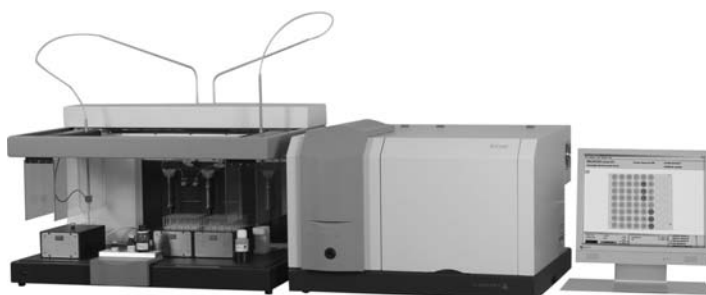
FIGURE 9.21 The D-Count microbial detection system based on flow cytometry. (Photo courtesy of AES-Chemunex, www.aeschemunex.com . With permission.)
