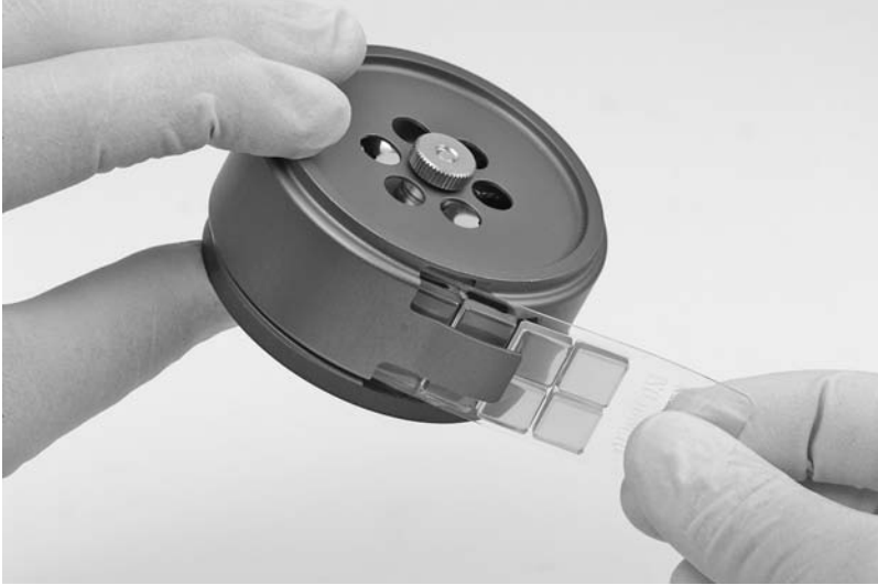
FIGURE 5.8 Insertion of agar strip in the RCS High Flow. (Photo courtesy of Biotest AG, www.biotest.de/ . With permission.)
