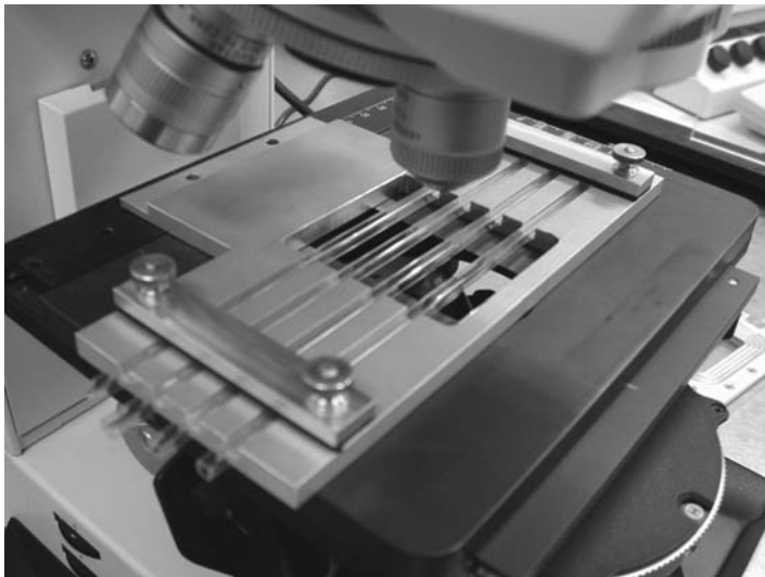
FIGURE 10.5 The Flow Cell System (mini-tube flow cell on microscope): a flat plate flow cell designed to accommodate coupons of various materials to study biofilms using microscopes. Other models are also available. (Photo courtesy of Paul Stoodley and Bryan Warwood, BioSurface Technologies Corporation, Bozeman. With permission.)
