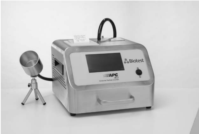
FIGURE 5.11 The APC M3 high-speed portable airborne particle counter. (Photo courtesy of Biotest AG, www.biotest.de/ . With permission.)
