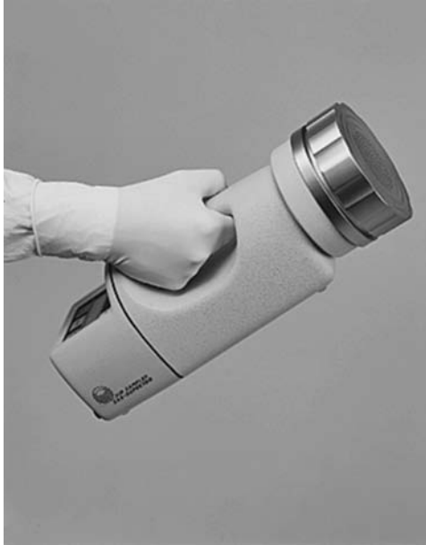
FIGURE 5.4 The SAS 180 air sampler. (Photo courtesy of Bioscience International, www.biosci-intl.com . With permission.)
